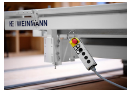
Pendant control panel (attached to the table flexibly) The control system is integrated into the table.
