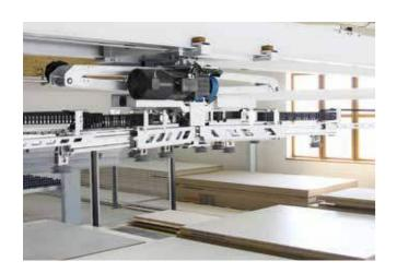
The ST71 suction cross rail in X geometry is the ideal optional feature for the panel storage. The self-learning cross rail generates the data required for panel handling independently and thus ensures dependable process reliability. The operator does not have to enter anything.
