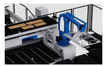
The system has a parts buffer directly above the pressure beam. This is where the robot temporarily deposits parts that are to be either destacked or fed to the saw again later.
