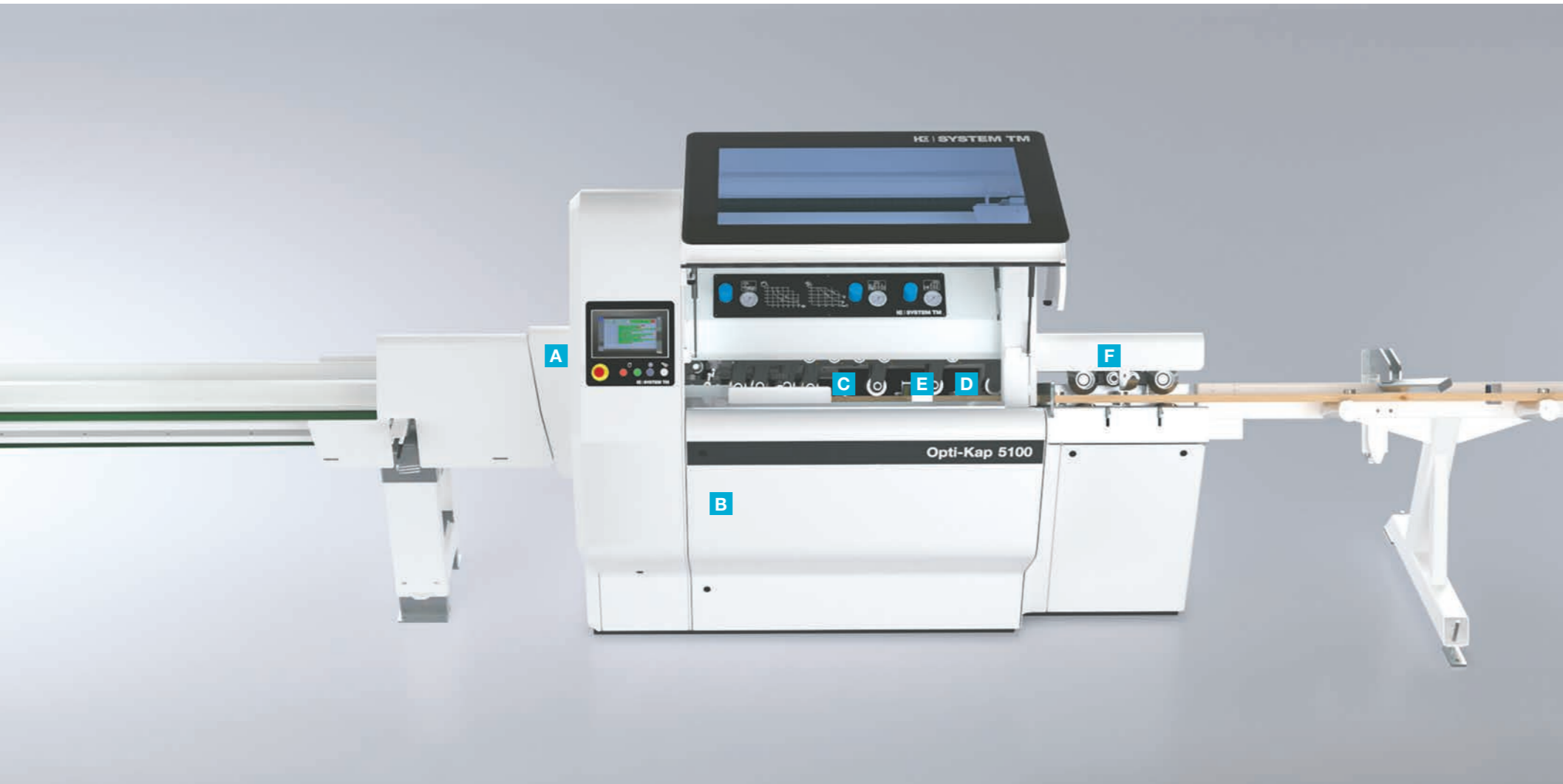
Integrated acceleration belt with driven fence for quick and exact positioning of workpieces that exit the saw.
