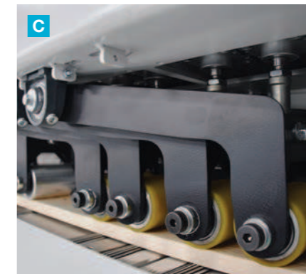
Heavy-duty infeed design with 9 driven bottom rollers and 9 top rollers. The rollers are supported on both sides to maximize and surface contact with each workpiece and provide excellent cutting accuracy.
