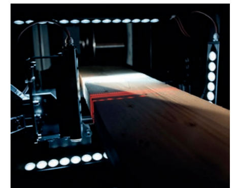
The Multi-Sensor scanning technology scans workpieces for best wood utilization.
