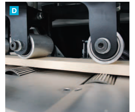
The bottom feed rollers are mounted high above the bed plate of the machine. This allows for the processing of bent and twisted timber, resulting in maximum productivity and cutting accuracy.
