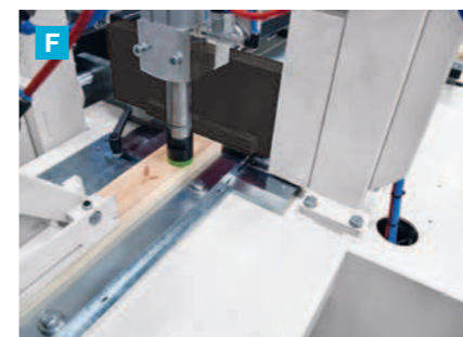
Cross-cut saw with fixed positioning of workpieces to pre-cut them into lengths before the press station.
