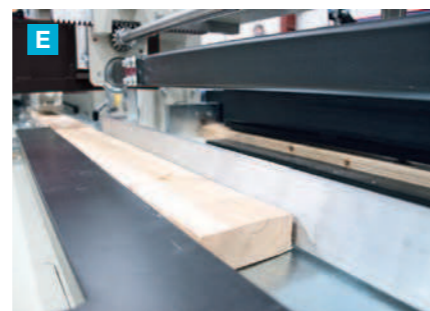
Two-channel press systems ensure high capacity. During the final pressing of workpieces, the work-pieces next in line are prepared for full utilization of the hydraulic press.
