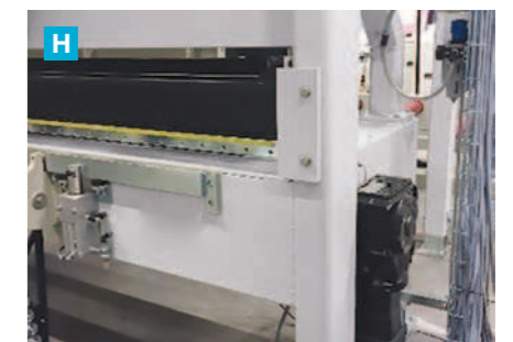
Heavy-duty pre-press and press frame to prevent deflection during operation.
