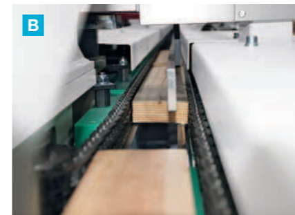
Pre-alignment and buffer zone. Two high-speed guide chains: one fixed and one moving. Top and bottom stainless steel guides ensure proper positioning of workpieces before pre-pressing.
