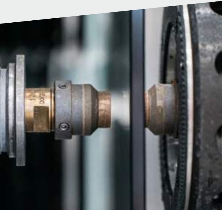
Drilling with two heads.
