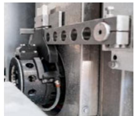
Dressing stick for dressing diamond grinding wheels and grinding device for polishing wheels.
