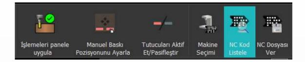
Integrated module to convert the applied toolpath into the language of the AES CNC machine.
