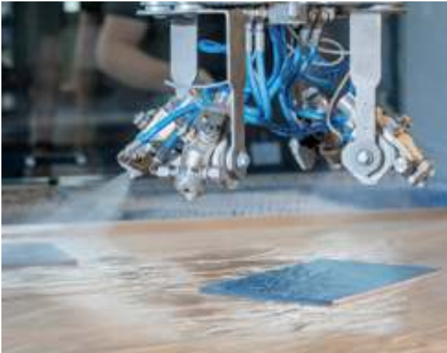
For automated painting. The SPRAYTEQ S-100 spray painting machine
