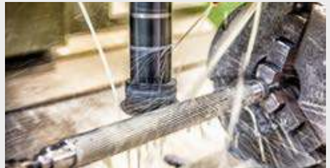
Milling of drive roll
