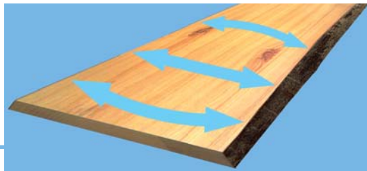
Fig. 22: Measurement and alignment of waney-edged boards in the automatic infeed system
