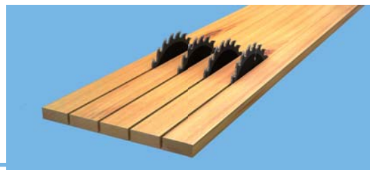
Fig. 25: Ripping of square-edged boards in the rip saw
