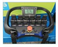
Multifunction control panel in operator friendly design with integrated buttons. Signal lights and Double action safety keys are both in the standard setup on the Winlet 350 TH.
