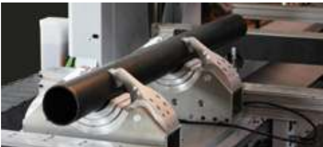
Clamping fixture for round pipes: Clamping fixture for 5-axis processing of round plastic pipes.
