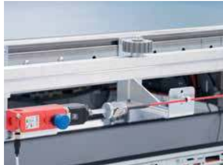
Equipment to achieve CE-conformity: rip cord back to the return belt
