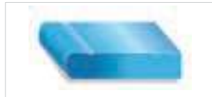
Pencil edge with grooving on the surface.
