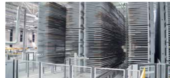
Collating between format and edge banding and drilling: Buffering and collating e.g. for assembly and tour order or color, form, dimensions etc..
