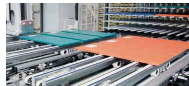
High storage capacity thanks to an ideal positioning of the material already in the entrance area: The material is exactly positioned while taken from the transport belt in order to fill the shelves ideally.
