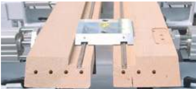
Clamping fixture for block frames: Precise clamping relative to the reference edge for a pair of block frames.
