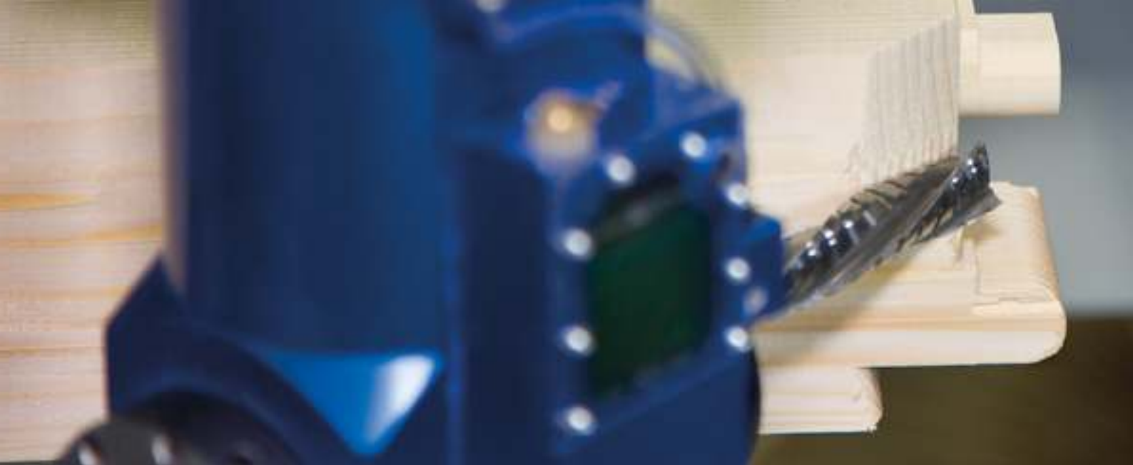
Traced flush trimming of edge overhang on postforming profiles.
