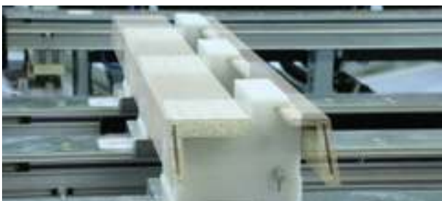
Clamping fixture for facings: Vacuum clamping fixture for a pair comprising rebate and ornamental facings according to customer design. Mounted on a base plate module.
