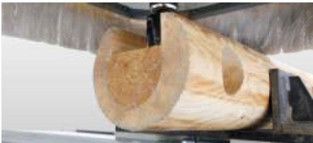
Block clamp: Adapted block clamping fixture for round timber elements.
