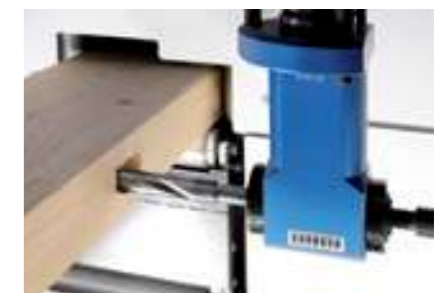
Production of mortises and pockets
