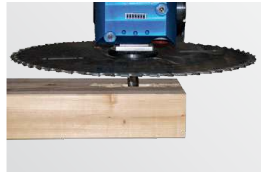
Saw blade with integrated routing unit
