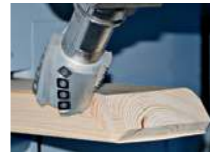
Producing a tenon joint
