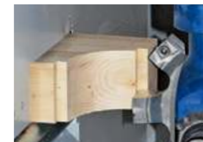
Machining the rafter head
