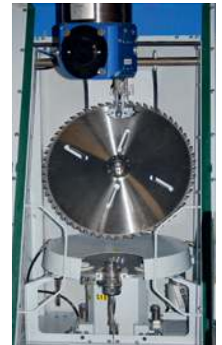
8-slot tool changer with pickup-station
