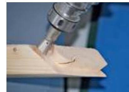
Dovetail at the jack rafter
