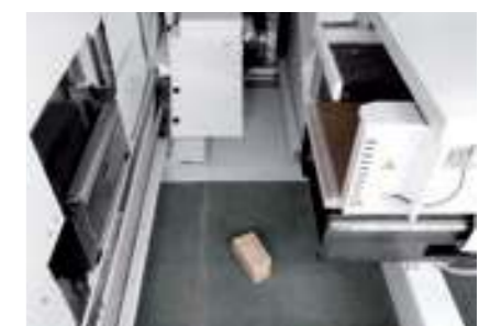
Conveyor belt with waste separation pusher is included in the base equipment
