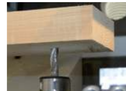
Milling a tenon hole with the underfloor unit
